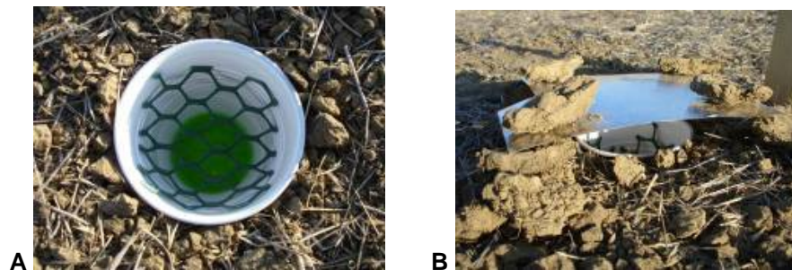
Figure 6. Pitfall trap viewed from above (A) and from the side with the aluminum cover (B).
